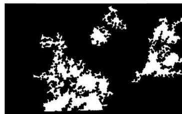
Fig. 14. Area Thresholding Applied to Filtered Image of Fig. 13
