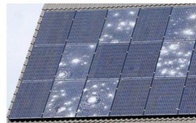
Fig. 8. Input Example Image of PV Panels with Hail Damage, cropped from the image in [14]
