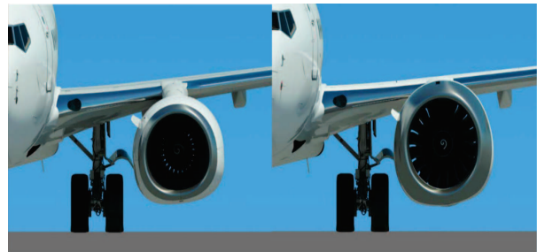
Fig. 1. New Leap Engine size on 737 MAX-8 (Right) vs. old engine on the 737 NG (Left) [4].
