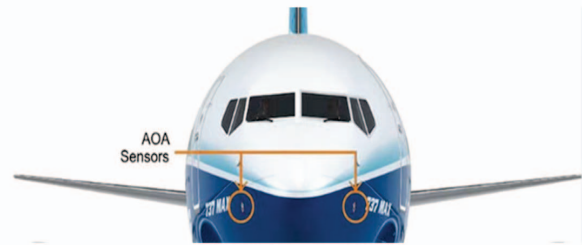
Fig. 3. AOA sensors location on the plane [1]
