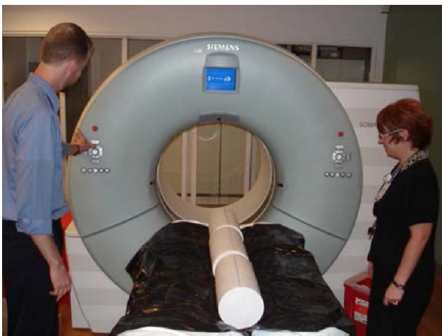
Figure 1. CT scanning of plaster specimen
